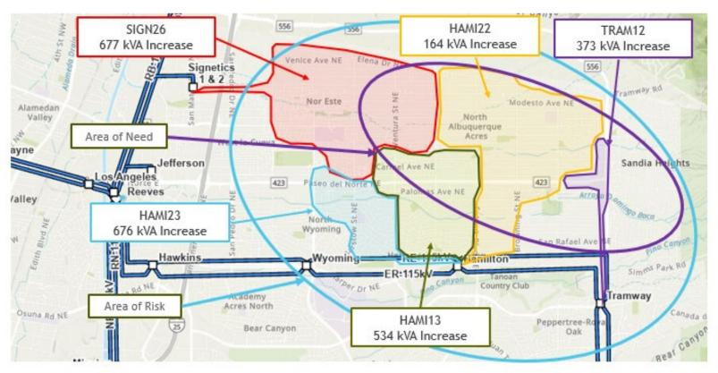
The colored areas on the map are the locations of load growth from 2021 to 2024. The load increase measured in each area is shown in kilovolt-amperes (kVA).
