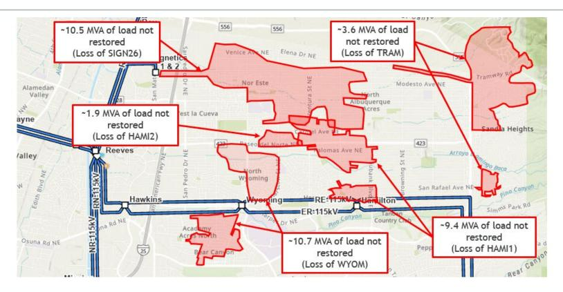
Projected 2031 potential areas at risk for brownouts in the event of a Substation Transformer outage during peak load timeframes.
