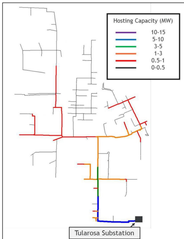
Figure 4-11: Example feeder hosting capacity heat map showing location-specific feeder constraints
