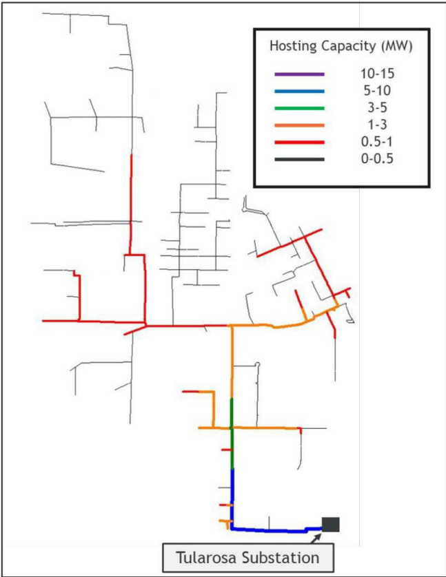
Figure 4-14: Example feeder hosting capacity heat map showing location-specific feeder constraints
