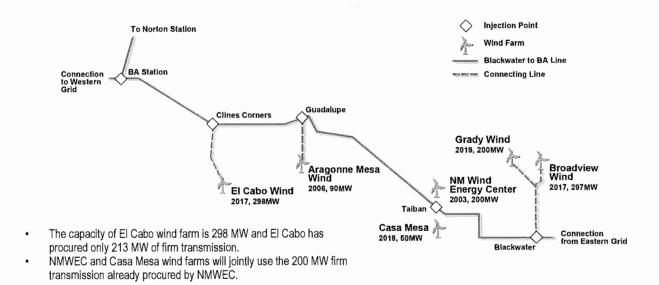
The BB Line runs from the BA 345kV Switching Station (BA Station) north of Albuquerque to the PNM Blackwater 345kV Switching Station (Blackwater Station) in the Clovis-Portales area of eastern New Mexico.
