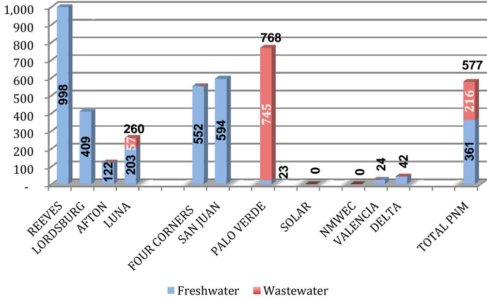
Figure 2-N illustrates the gallons consumed per MWh, also known as water intensity, by PNM’s current generation plants.
