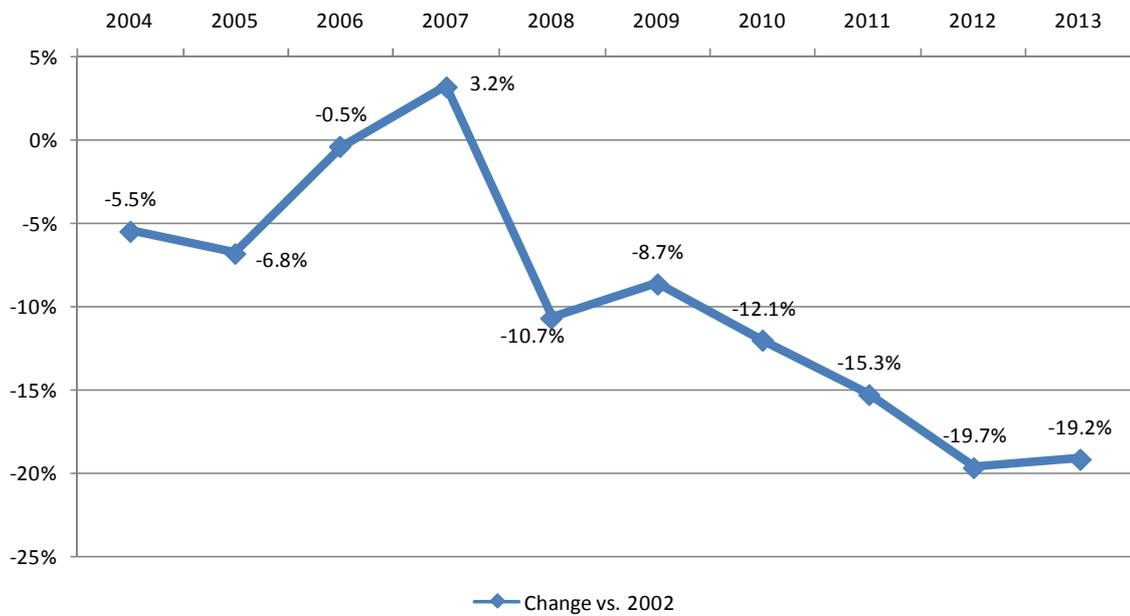
Water usage at PNM's generating facilities vary from year to year due to many different factors such as weather, capacity factor, load factor, leaks, water quality variations, and the availability or ability to use gray water. Nevertheless, water use on a total portfolio basis has been generally declining since 2002, as shown in Figure 2-N, above. For example, the average water intensity of PNM's generating portfolio in 2013 was 19% lower than the intensity during 2002.
