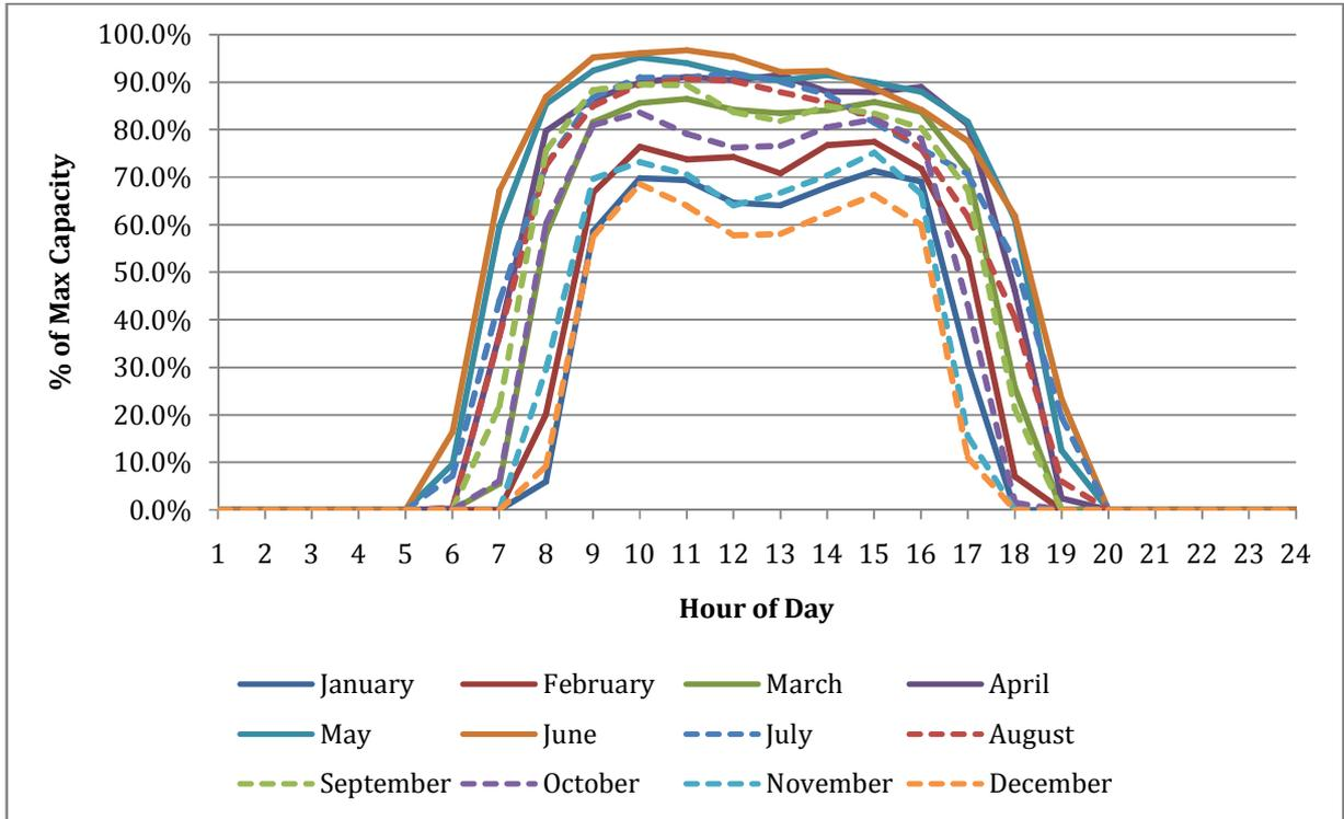
The energy production curve from July was used to define the effect of solar PV contribution on PNM’s system peak. July is the month when PNM is most likely to see its annual system peak demand and the hour that corresponds with the peak is normally 4pm or hour 16. The production curve is shown below in Figure 6-T. As shown in Figure 6-T, the solar PV peak contribution at the peak hour is approximately 76%.
