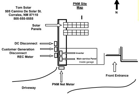
REC meter & Net Meter are not grouped together and not in plain line of sight Site Map is placed at the PNM Net Meter. 1-line diagram is placed at the REC Meter.
