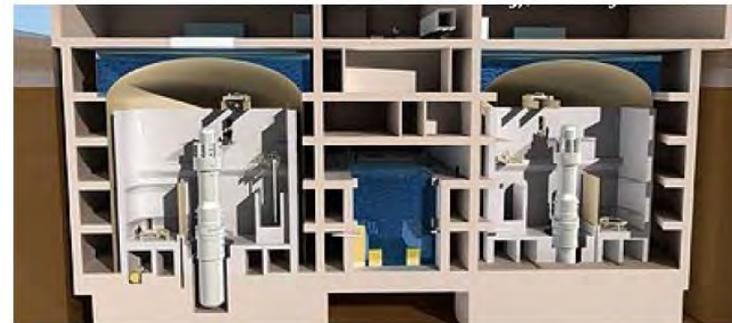
Figure 4-2. Conceptual drawing of an underground containment housing two B&W mPower reactor modules
