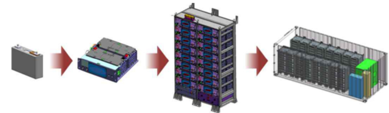
Figure 5. Structure of a Li-ion System
