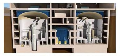
Figure 4-2. Conceptual drawing of an underground containment housing two B&W mPower reactor modules Source: B&W Nuclear Energy
