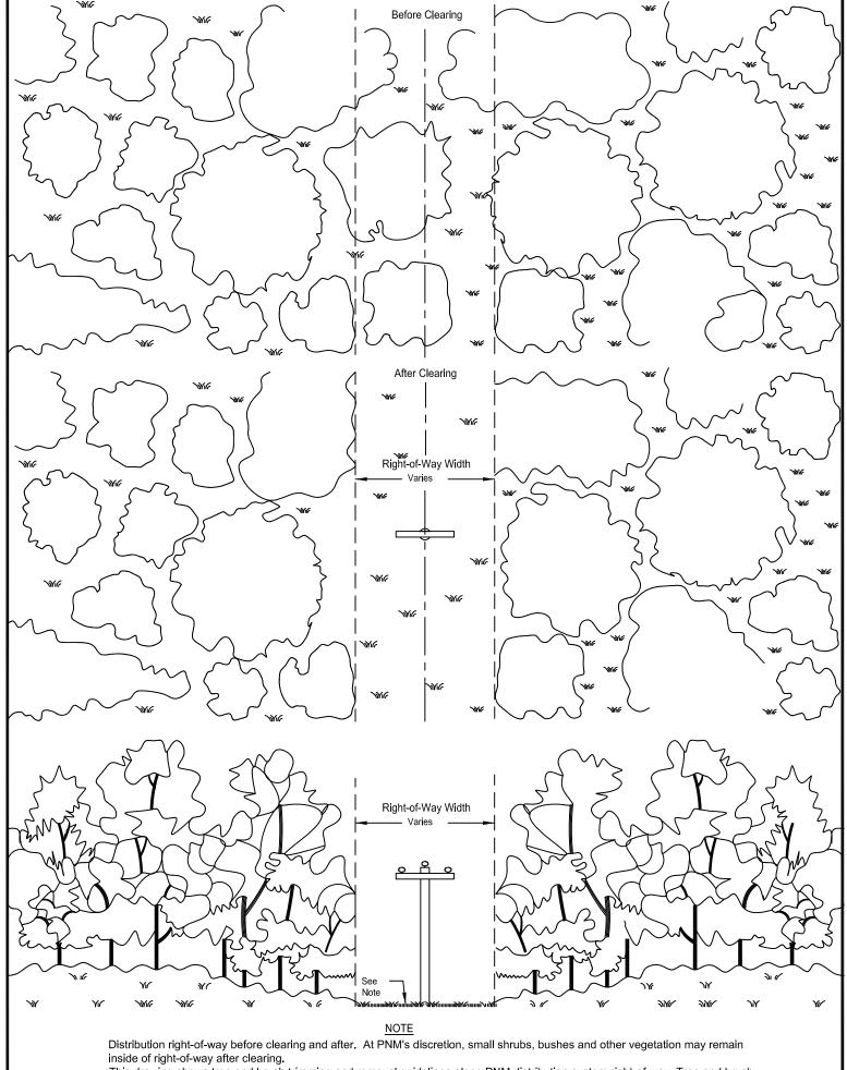
This drawing shows tree and brush trimming and removal guidelines along PNM distribution system right-of-way. Tree and brush trimming and removal are important to help ensure PNM electrical delivery system reliability.
