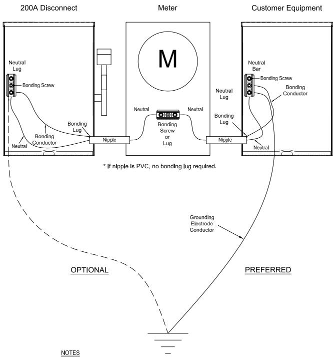
(1) In some cases such as switchgear, meter packs, pedestals, temp services, etc. the drawings may not apply due to how things are manufactured. These would fit for most single meter, self-contained services.
